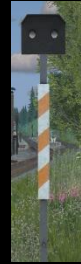
So 18 – Monitoring signal of the dropout (only optical, the Train Simulator cannot display dropouts)
