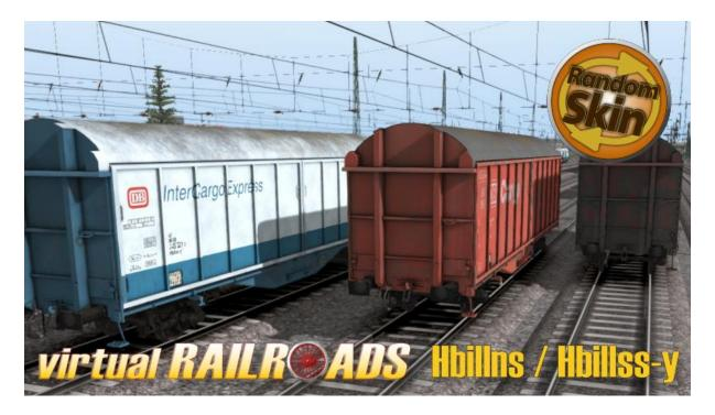
Two-axle sliding wall wagon used for the transport of moisture sensitive goods.
